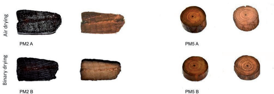
Figure 4. PM2 samples A and B. On the left the wet sample and right the sample after drying. And PM5 samples A and B. On the left the wet sample and right the sample after drying.
