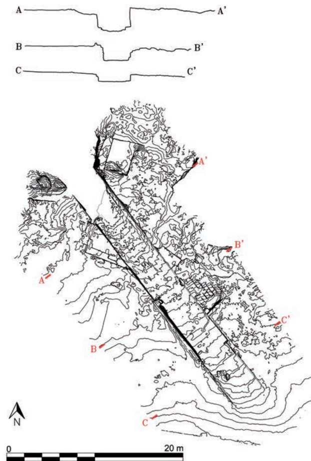
Figure 2. Detailed plan of the slipway and three cross sections.
