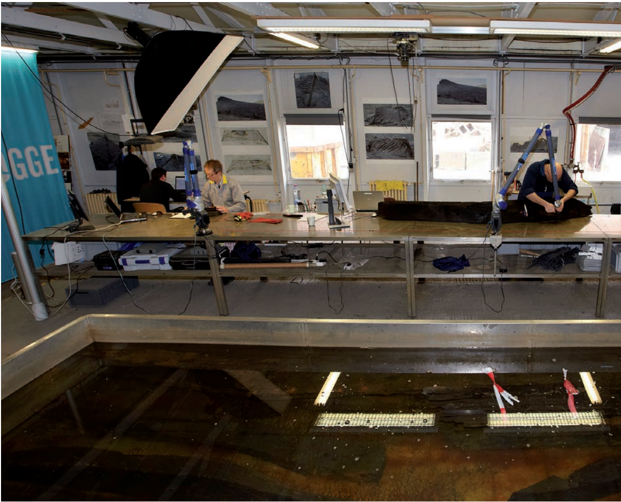
Figure 4. The Doel Ships research laboratory. With FRAUG techniques and Faro measuring equipment, more than 900 pieces of timber were analysed. ©Kris Vandevorst Onroerend Erfgoed.
