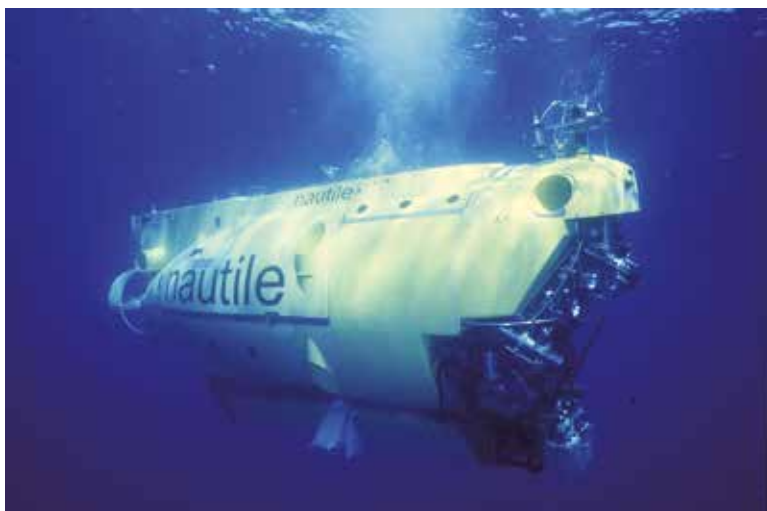
Fig. 1 – The Nautilus , a manned Ifremer submersible, designed for observation and intervention at depths of up to 6000 m. © Ifremer / É. LACOUPELLE. ■
