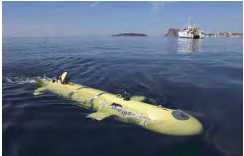
Fig. 2 – The AUV Aster X (IFREMER), an autonomous vehicle weighing around 800 kg, which can descend to depths of up to 3000 m. © Ifremer / O. DUGORNAY. ■
