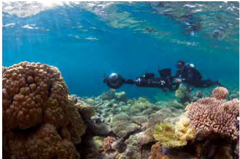
The XL Catlin Seaview SVII camera in action, in the Maldives in 2015. It allows the collection of 360° images every 3 seconds, travelling at a speed of 4 km/h. © The Ocean Agency / XL Catlin Seaview Survey / C. BAILHACHE. ■
