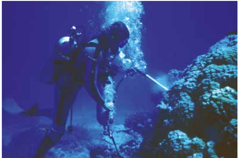
Fig. 2 – Extraction of a core using a manual pneumatic pressure drilling technique (Wheeler Reef, Australia). © L. MONTAGGIONI / CNRS Photo library. ■
