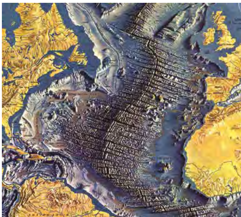
Fig. 1 – North Atlantic undersea relief, from the 1977 physiographical map by Marie Tharp and Bruce Heezen. This map, based on bathymetric profiles, shows the mid-ocean ridge split by transform faults, and numerous volcanic seamounts. ■
