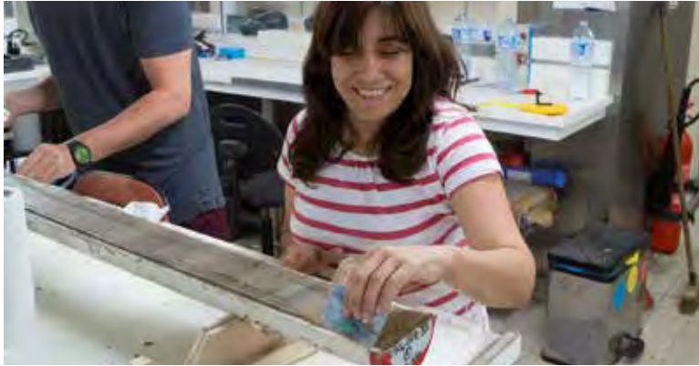
Fig. 2 – Preparation of an ocean sediment core for the purpose of description and analysis. © E. MORENO – CASEIS campaign the vessel Pourquoi pas ? ■
