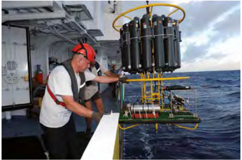
Fig. 2 – Launch of the CTD rosette bathymetric sounder from the oceanographic vessel L'Atalante. © S. LESBATS / Ifremer. ■
