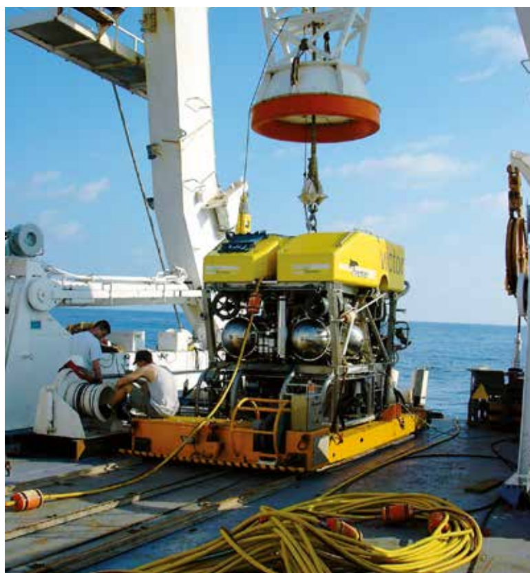
Fig. 1 – The manned Victor 6000 ROV, shown here during a maintenance operation on the rear deck of the oceanographic vessel Atalante, is a remotely operated underwater vehicle designed for oceanography research. The lower part of the vehicle can be adapted to suit the needs of the specific assignment and is equipped with scientific instrumentation. It is capable of working at a depth of 6,000 metres. © J.F. TERNAY / CNRS Photo library. ■
