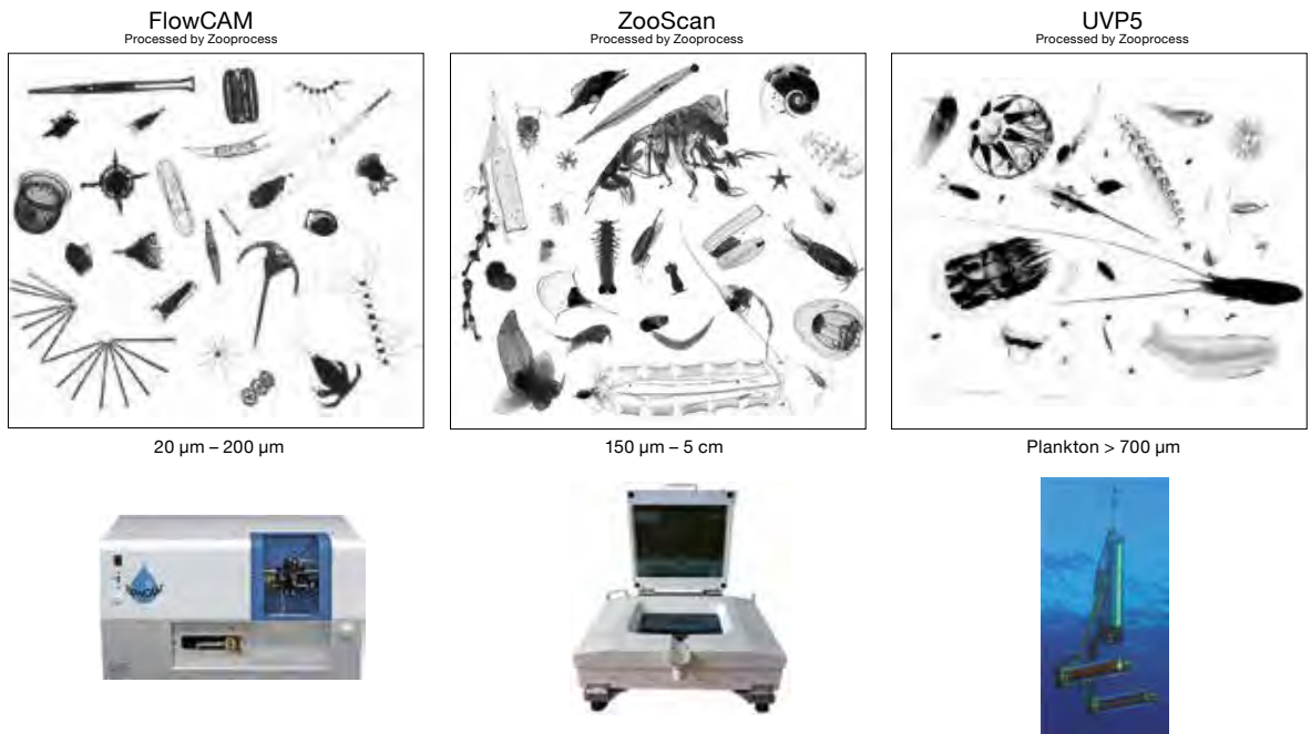
Fig. 2 – Left to right: thumbnail images of microplankton organisms imaged with FlowCam, mesozooplankton organisms imaged with ZooScan, and macroplankton organisms recorded with the Underwater Vision Profiler (these two instruments are distributed under CNRS license). Zooprocess is an open source image acquisition and processing software designed by M. Picheral of the LOV. © A. ELINEAU, Observatoire Océanologique de Villefranche-sur-Mer. ■
