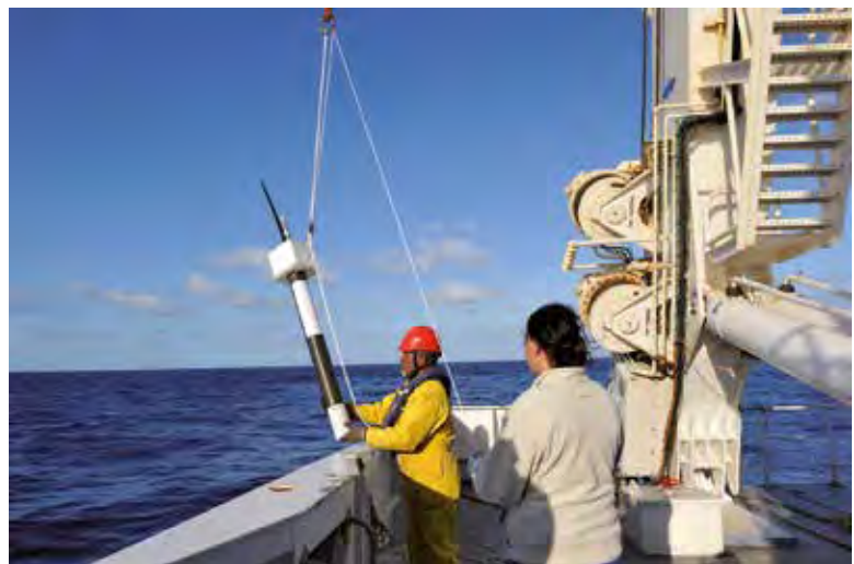
Fig. 1 – Example of the deployment of an Argo float. Argo floats are deployed in all oceans, from research vessels, ships of opportunity and sailing boats. © Ifremer. ■
