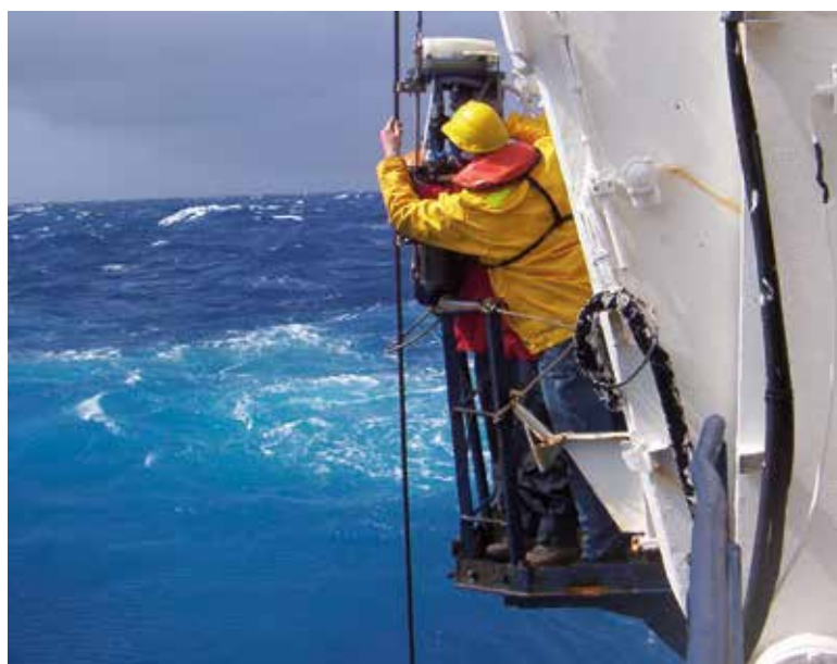
Fig. 1 – Lowering of a pump allowing sea water filtration, from the ship Marion-Dufresne . © M. SOUHAUT. ■
