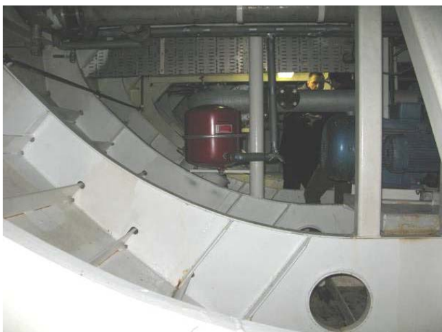
Figure 3. In the foreground envisaged installation place of APS. In the background seawater pipe with flange for re-introduction of APS water into the ship's seawater system.
