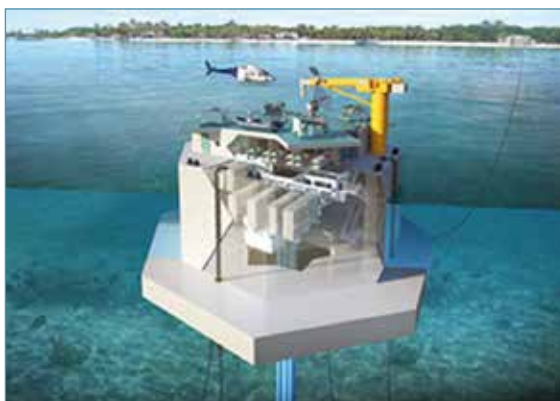
Offshore 1 MW OTEC
