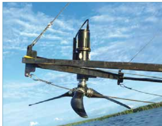
Successful development & deployment of a barge based tidal turbine by ERI@N along with its industrial partners: Schottel Hydro, Ocean-Pixel, Aquatera.
