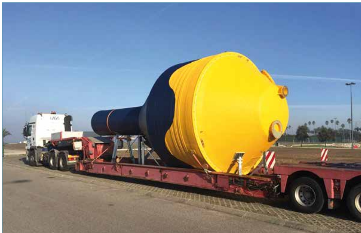
Stage 3 of CorPower's device (in composite hull)
