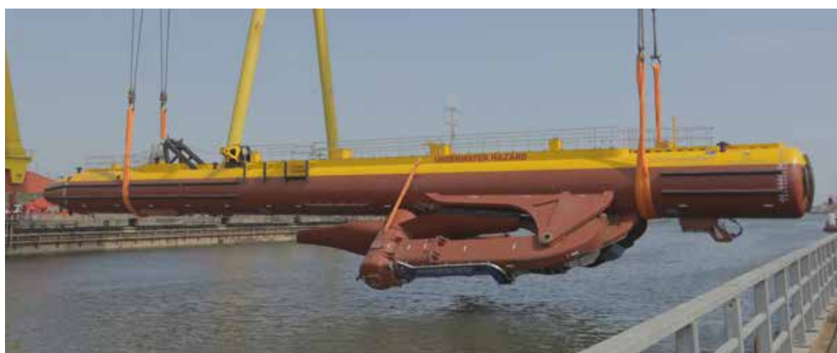
Scotrenewables Tidal Power tidal turbine at Harland & Woolfe Shipyard, Belfast
