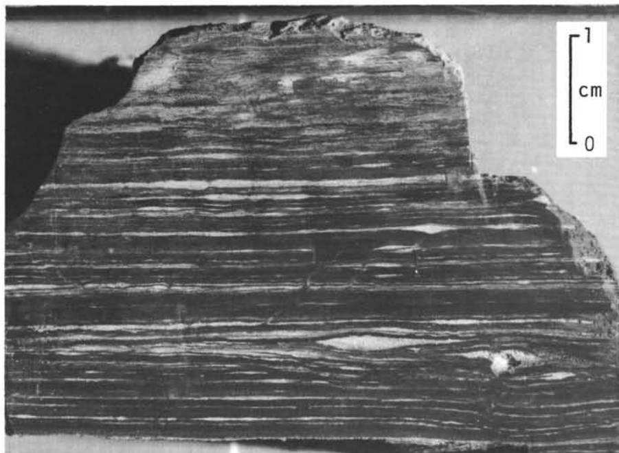
Figure 4. Probable "contourite" silt laminae, 268-17-3. Note lenticularity of laminae, erosional scours not filled with coarser silt, and slight bioturbation.
