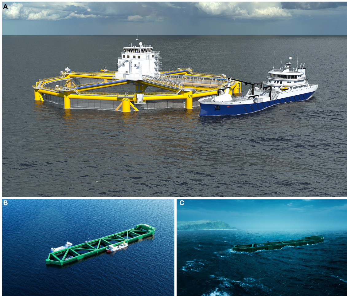
FIGURE 5 | (A) Large offshore fish farm device with a diameter of 110 m, a height of 67 m and a volume of 245,000 m 3 (upper image). This fish farm was just recently built in an Asian shipyard, transferred to Norway and could produce 6,000 t of salmon. (B,C) Havfarm 1 : Large aquaculture production unit integrated into a vessel-like floating platform in calm (lower left) and rough (C) conditions at sea (lower right). Havfarm 1 includes next to the large cages a mini-harbour for service vessels, maintenance trolleys along the outer rails providing access to the entire facility, rotatable thrusters to reduce stress on the mooring during storm conditions while also ensuring optimum oxygen supply, and a deep steel louse skirt, which reduces the risk of lice infection as well as protects the facility from being damaged by drifting objects [Image (A) with permission of NSK Ship Design and image (B) with permission of Ocean Farming AS].
