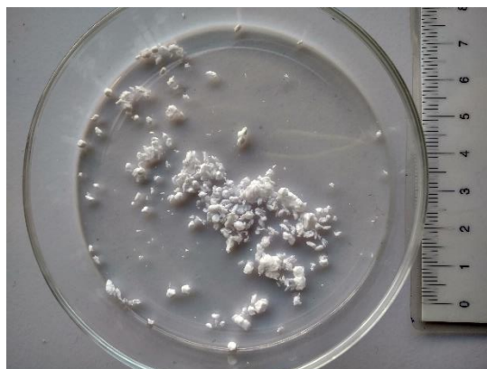
Figure 6 – EPS pellets obtained after grinding procedure (ranging between 1-4mm)
