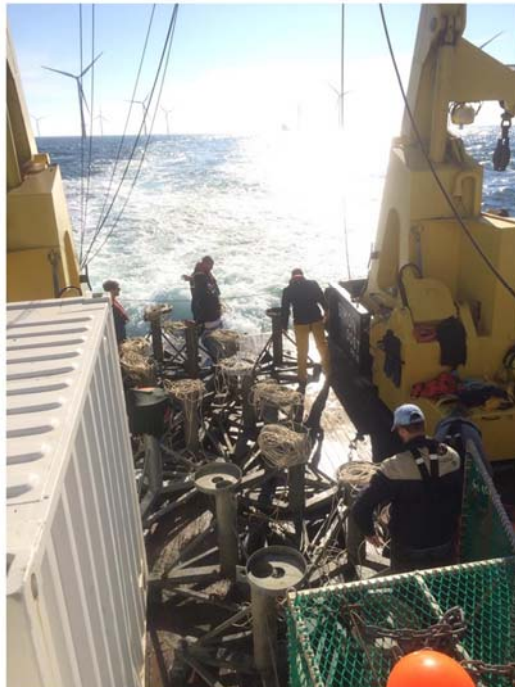
Fig. 1: a) AZFP mooring device, including two acoustic transducers (38 kHz and 125-200-455 kHz, which was 125-200-455 and 769 kHz for the second one), battery pack and pop-up acoustic release assembly. This mooring was lowered to the seabed using a large A-frame for handling. Image taken from manual AL-77E01F00-R03-PR936, ASL Environmental Sciences Inc. b) The two AZFP-echo sounders on deck of the RV Simon Stevin of the Flemish Government before deployment c) deployment of equipment with the A-frame.
