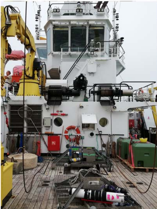
Fig. 1: a) AZFP mooring device, including two acoustic transducers (38 kHz and 125-200-455 kHz, which was 125-200-455 and 769 kHz for the second one), battery pack and pop-up acoustic release assembly. This mooring was lowered to the seabed using a large A-frame for handling. Image taken from manual AL-77E01F00-R03-PR936, ASL Environmental Sciences Inc. b) The two AZFP-echo sounders on deck of the RV Simon Stevin of the Flemish Government before deployment c) deployment of equipment with the A-frame.
