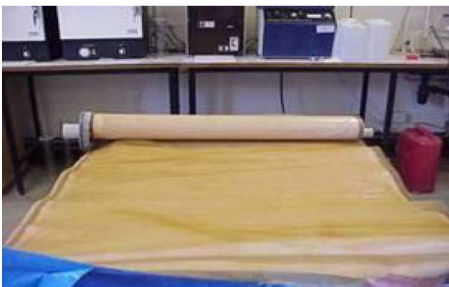
Figure 5 | Autopsied SW membrane associated with a fouled product hose.
