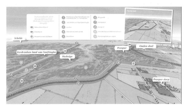
To accomplish the above, a new inland dike of 4,7m is being constructed, an average of 9m above ground level (+12,50m TAW) with a 80m wide foundation and a top width of 7m. The centre of the dike is build with sand (900.000m³) which is mainly delivered over water by the Client Waterwegen &
