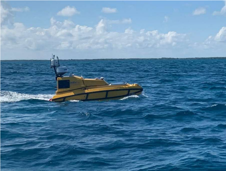
Figure 16: The CAMEL Autonomous Surface Vehicle (ASV), C-Worker-4
