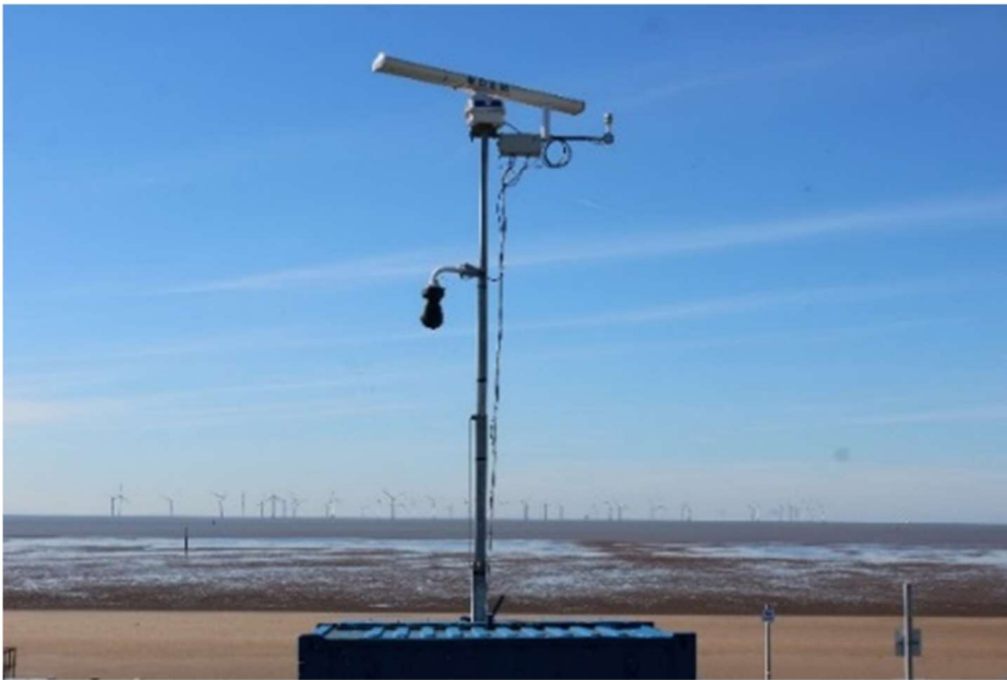
Figure 13: Radar survey platform (Marlan Maritime Technologies Ltd)
