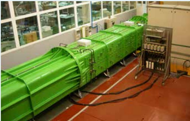
Figure 19. The SEA-TITAN project is developing a second-generation Direct Drive PTO (first-generation PTO in the picture).
