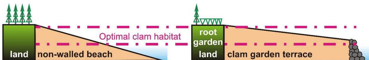
Fig. 4. Sectional schematic illustrating the basic architecture of a clam garden. The structure of the clam garden (at right) is compared with the profile of the original beach (at left). Clam gardens were often accompanied on the landward side by root gardens, which were tended for a variety of plants and edible bulbs and where shrubs and trees were pruned, and even nourished, to increase berry and fruit production. Redrawn and adapted from Groesbeck et al. (2014) and Wyatt (2015).
