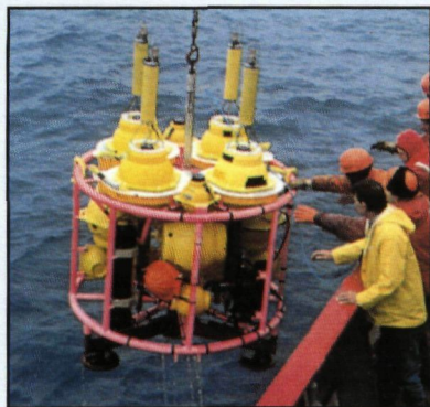
Deployment of deep sea pressure recorder with releasable data capsules.
