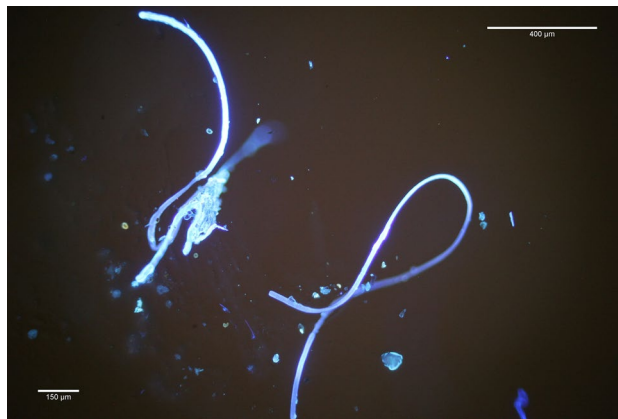
Figure 2. Microplastic fibres and particles under the microscope. Each of the filters collected was inspected and investigated under the microscope to quantify the amount of microplastic fibres and particles. Most polymers, the main structural molecular blocks of plastics, tend to shine under the ultraviolet light (UV-light), which was done using a BX53 Olympus microscope.
