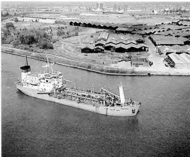
Fig. 68 — Towed hopper suction dredger "Khersones".
