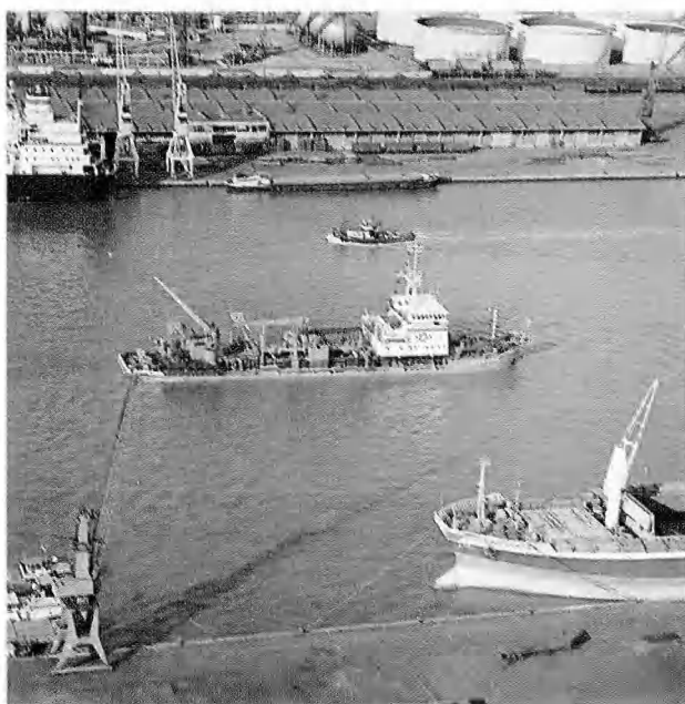
Fig. 66 — Towed hopper suction-dredger "Krankeloon".
