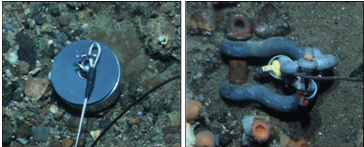
Figure 5: Examples of the lead weight (left) and interlocked shackles (right) used in the 1-cm scale bar calculations for the 2015 Stone Fence image analysis.
