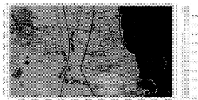
Fig. 8 Isopleths plot of the predicted daily average ground level concentration of PM
