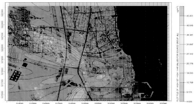
Fig. 7 Isopleths plot of the predicted hourly average ground level concentration of PM
