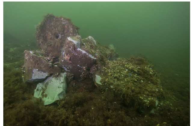
Fig. 3 Chunks of hexanite (German Schiesswolle) with starfish, mussels and other kind of marine fouling on the surface © Jana Ulrich, FTZ CAU
