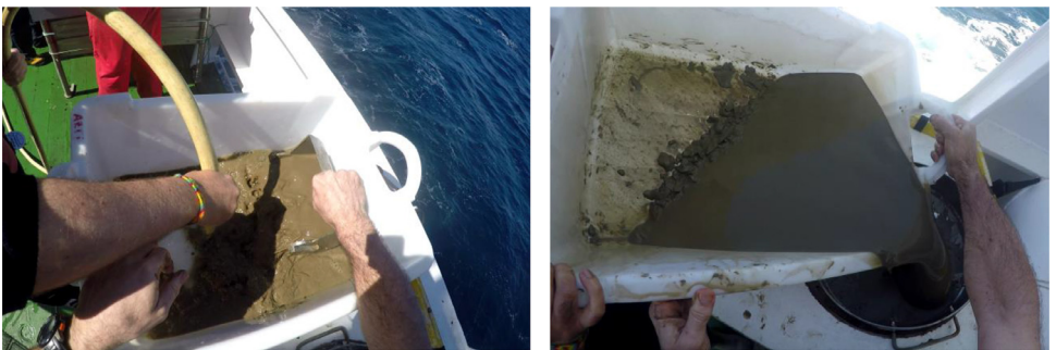
Fig. 5. Sieving of sediment through a 1 mm mesh size sieve, for the separation of macrofauna.
