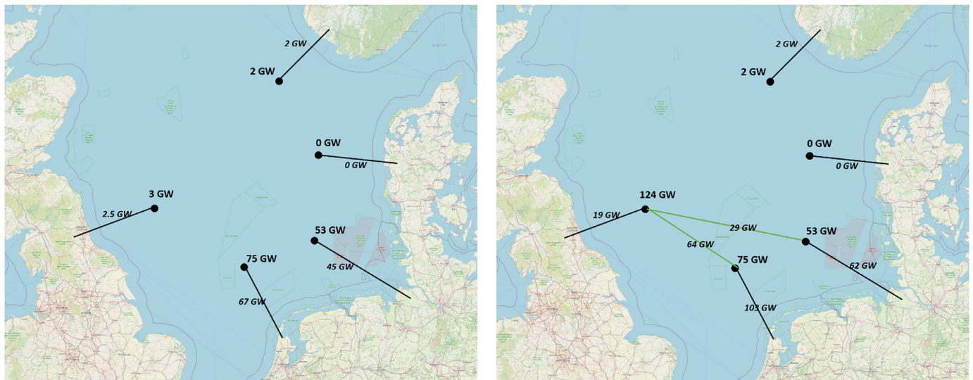
Fig. 15. Installed capacities and HVDC interconnectors deployed in the scenario HVRE.
