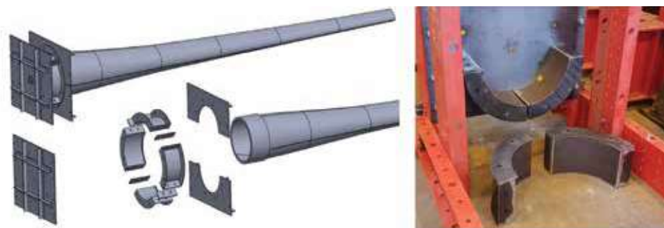
Figure 4. Design for the torsion box root connection.
