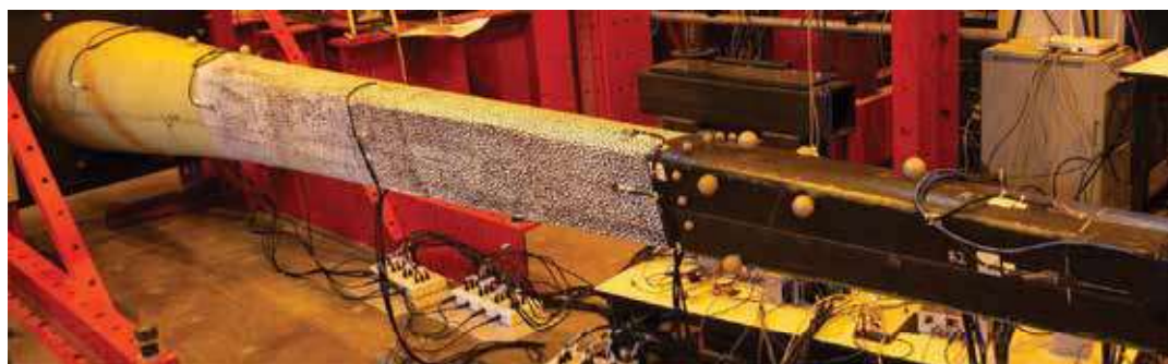
Figure 5. Test setup showing transition area covered in white paint and speckling pattern for DIC.
