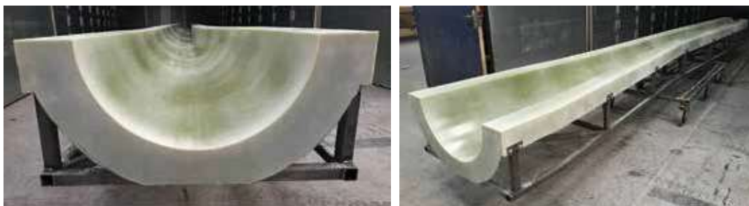
Figure 1. Blade mould half after curing.
