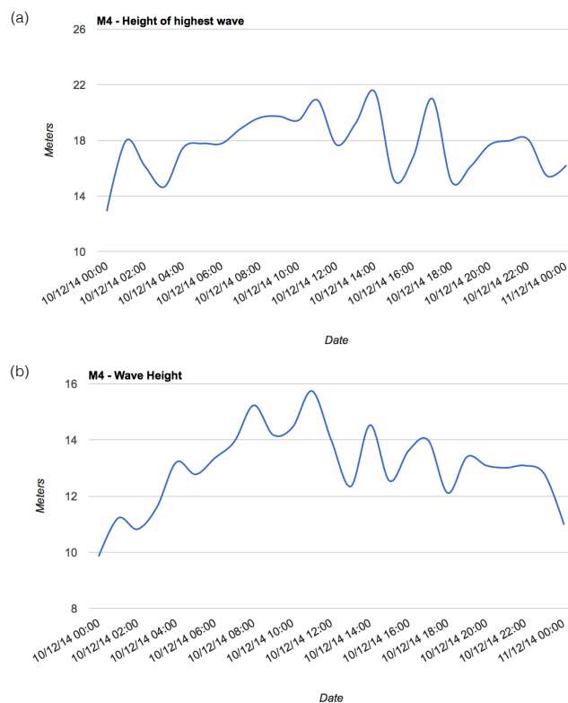
Figure 9. M4 records of (a) maximum wave height (m) and (b) significant wave height (m) on the 10th December 2014.
