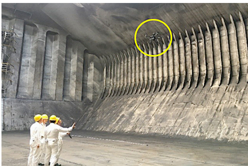
Figure 13. Drone flying inside the cargo hold by ClassNk. Source: gcaptain.com
