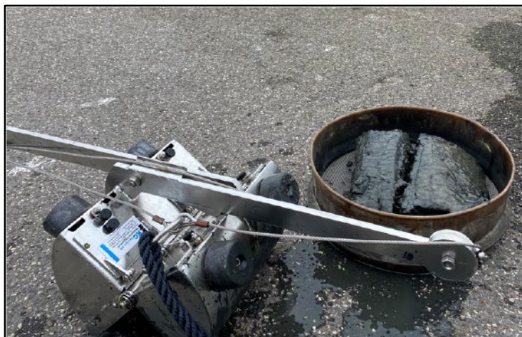
Figure 2.3. Van Veen grab and sieve used for sediment sampling
