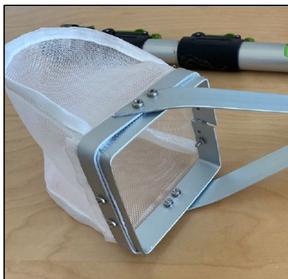
Figure 2.4. Scraper used to collect biological material on hard substrates in the harbors.
