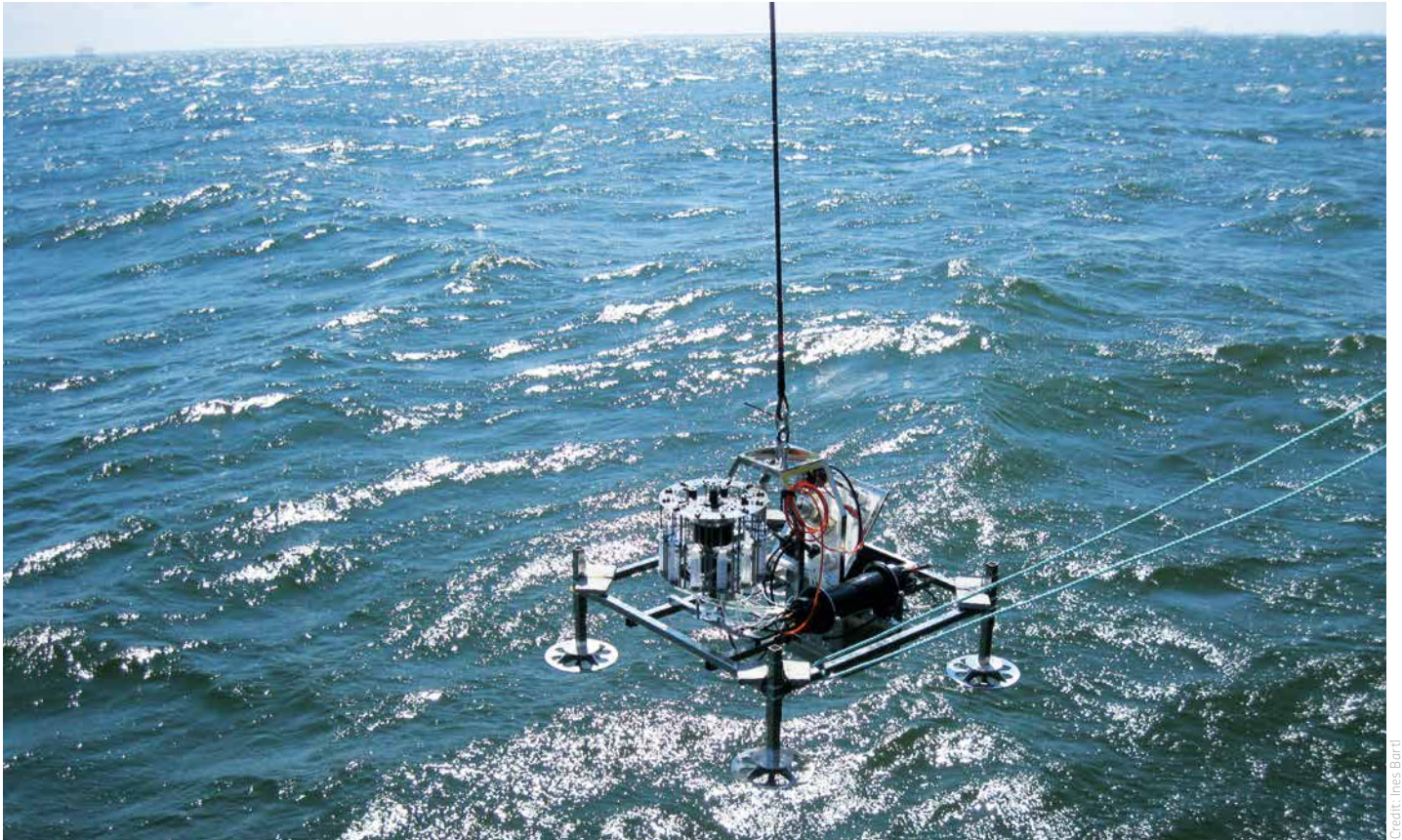
Figure 5.4 A benthic lander being deployed from a ship. Benthic landers are observational platforms that sit on the seabed to record physical, chemical or biological activity.
