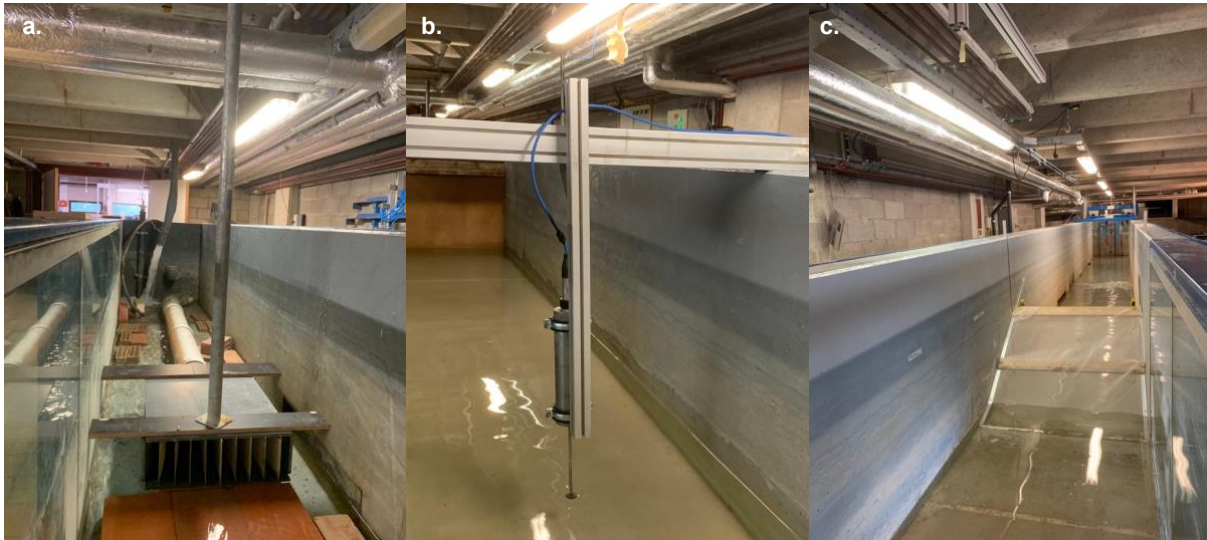
Figure 2. Some components of the artificial flume setup. (a) Inlet of water in the flume. (b) Valeport 802 electromagnetic current flow sensor. (c) Installed screen near the end of the flume to trap samples that escape the catcher.
