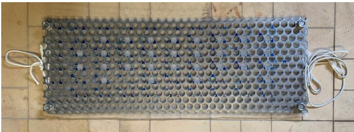
Figure 4. Image of the customized made loading plank, to insert plastic debris and reeds into the mesocosm setting.
