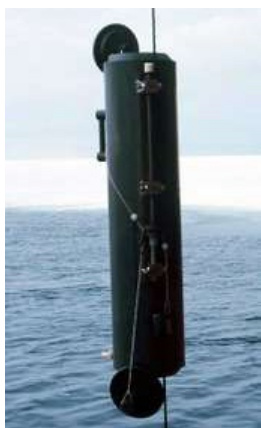
Figure 4. Niskin bottle for sampling the water column at a certain depth.
