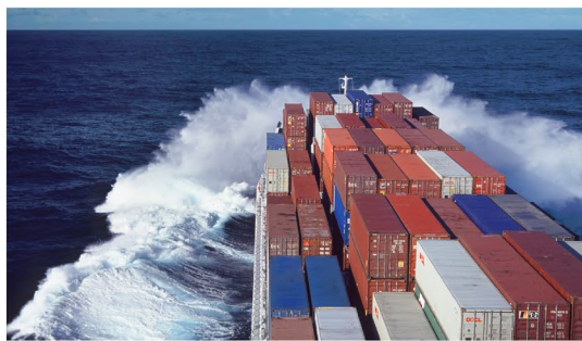
(a) Photo from the bridge of the considered vessel; a 2800 TEU Panamax container ship.
