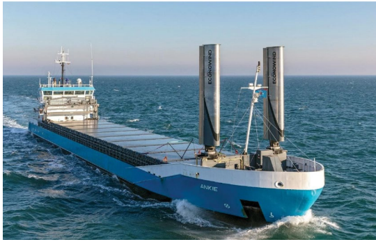
(a) Onboard decision support for wind-assisted propulsion. With permission by ECONOWIND ( www.econowind.nl ).
