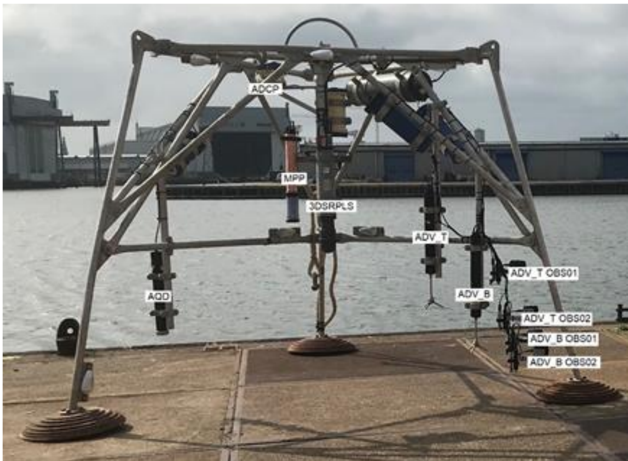
Figure 6: Frame containing all the measuring instruments.
