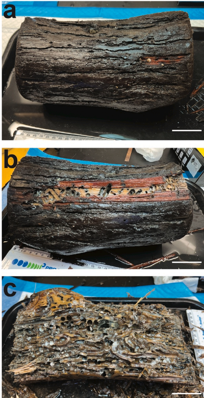
Fig. 1. Bald cypress log deployed at the Alabama Undersea Forest site for eight months. (a) Undissected log, (b) log with a portion of the bark removed exposing empty shipworm burrows near wood surface, (c) dissected log exposing crowded shipworm burrows within the interior of the wood. Scale bar, 5 cm.
