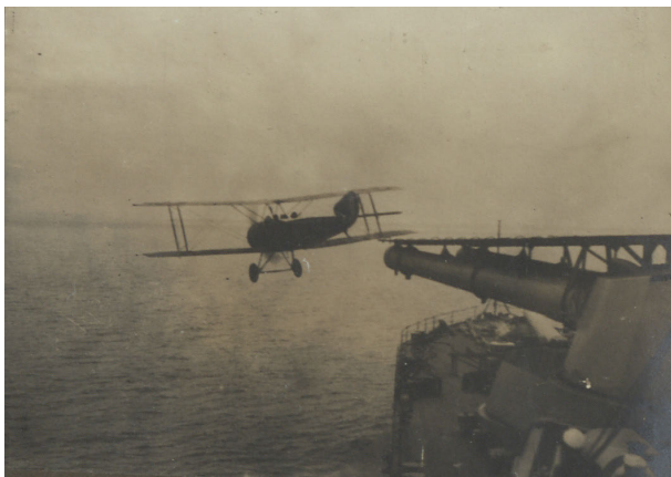
FIGURE 3. Plane flying off turret of HMS Barham (~ 1918) (Courtesy national museum of the royal navy).
