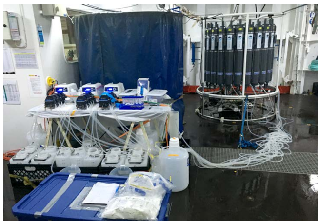
FIGURE 3. Typical oceanographic eDNA collection strategy. Seawater in Niskin bottles on a CTD rosette is filtered for eDNA collection. In this example, tubing connects the Niskin bottle spigots directly to filters with submicron pore sizes. Seawater is pumped with multi-head peristaltic pumps so that several samples can be filtered simultaneously. The filtering outflow is collected in carboys to determine the exact volume of water filtered. Photo credit: Erin Frates (WHOI)
