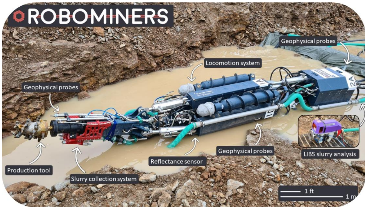
The ROBOMINERS "RM1" prototype during the July 2023 tests in the Kunda mine, Estonia
