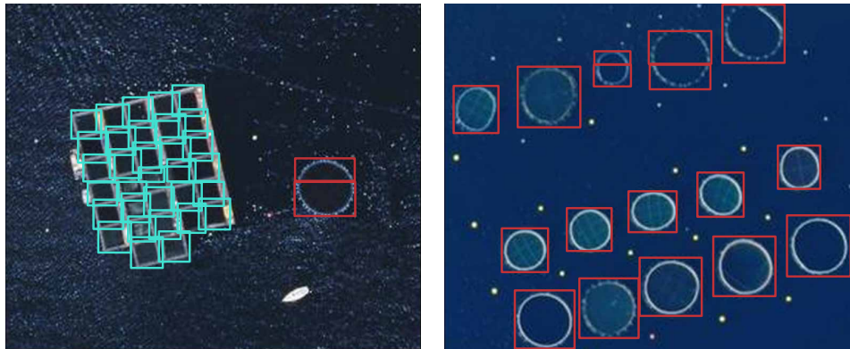
Fig. 2. Example detections of aquaculture cages. Detections of surface square (cyan) and circular (red) finfish aquaculture cages identified by our object detection model on aerial imagery of the French Mediterranean. Imagery: IGN (42).
