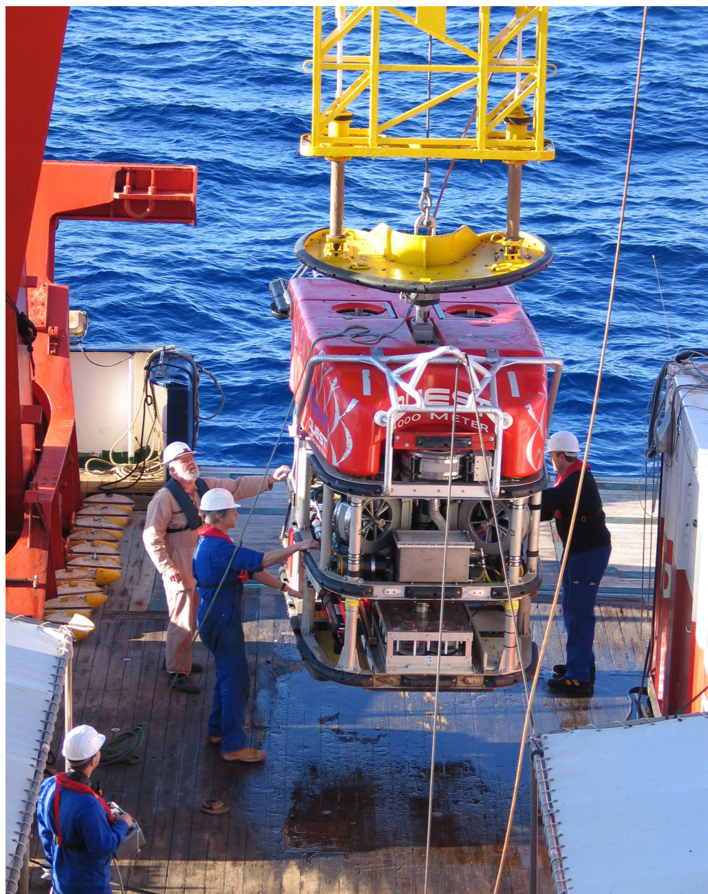
Use of the ROV MARUM-QUEST from the research vessel METEOR during an expedition in the eastern Mediterranean
