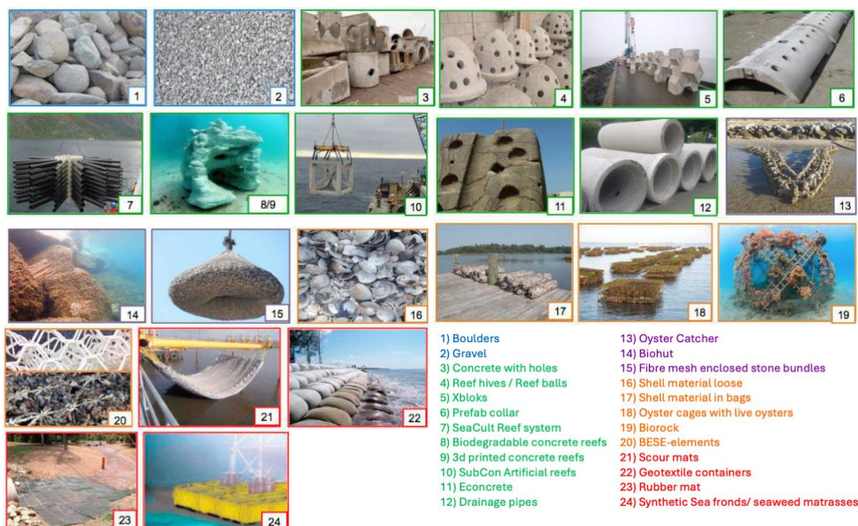
Figure 17. Materials used for scour protection. Blue is conventional scour protection material, green represents large structures that provide holes, purple shows smaller structures to increase complexity, orange shows natural substrates, and red is materials made of plastics. Adapted from Lengkeek et al. (2017).
