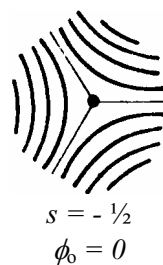
Fig. 22. (a) Identification of the angles \phi and \theta_r used to describe a disclination. (b) Director arrangement of an s = \pm 1/2 singularity line. The end of the line attached to the sample surface appears as the point s = +1/2 (points P). The director alignment or field does not change along the z direction. The director field has been drawn in the upper and the lower surfaces only.
