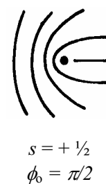
Fig. 22. (a) Identification of the angles \phi and \theta_r used to describe a disclination. (b) Director arrangement of an s = \pm 1/2 singularity line. The end of the line attached to the sample surface appears as the point s = +1/2 (points P). The director alignment or field does not change along the z direction. The director field has been drawn in the upper and the lower surfaces only.
