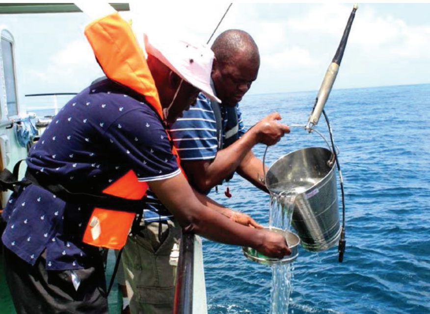
Plate 5.1.2: Sieving of surface phytoplankton using a 20 litre bucket
