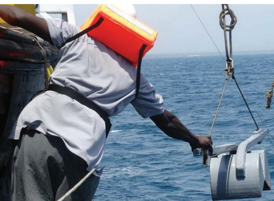
Plate 5.1.3: Sampling of benthos using a Van-Veen grab sampler attached to a winch
