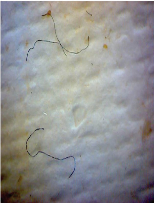
Plate 5.9.1: Microplastic filaments obtained from digested zooplankton in Kenya's marine water (x40 magnification)
