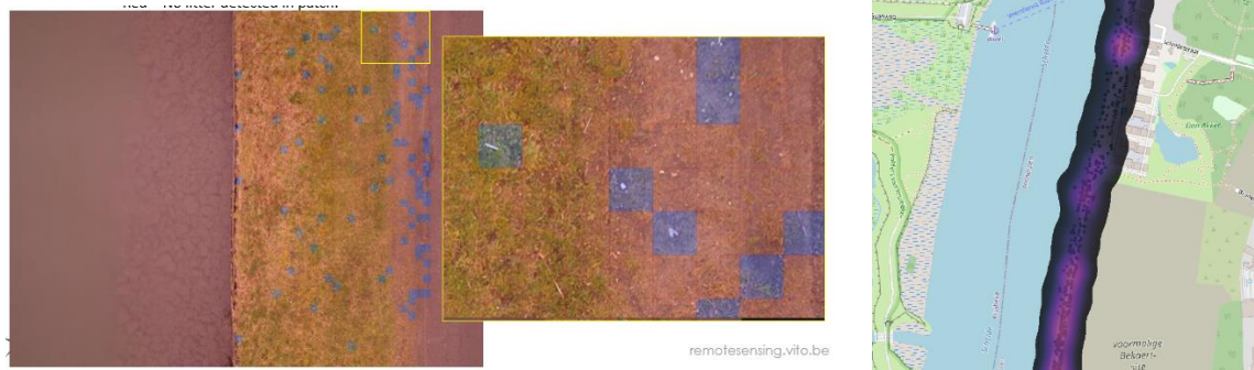
Fig. 12. Left: Patches of litter identified from drone data. Blue patches indicate presents of plastic items > 2.5cm, red coloured patches are areas not polluted by litter. Right: shows a derived waste map, showing hotspots of litter along the riverbank.
