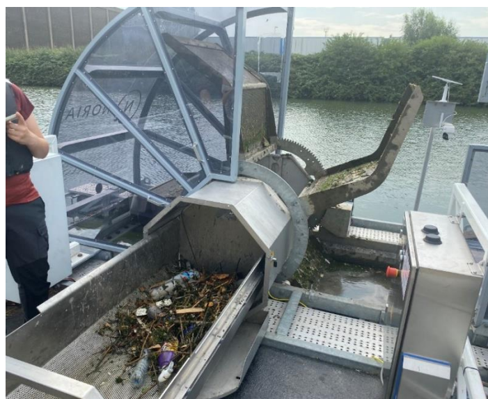
Figure 32: CirCleaner's collection compartment (Photograph by Jan Puhar).
