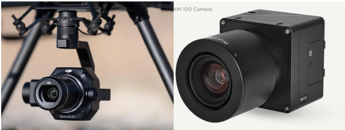
Figure 3: Image of Zenmuse P1 (left) and Phase One iXM-100 (right) camera (Phase One, 2024).
