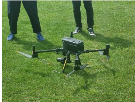
Figure 2: Matrice 350 RTK drone platform (photograph by Mariana Miranda).
