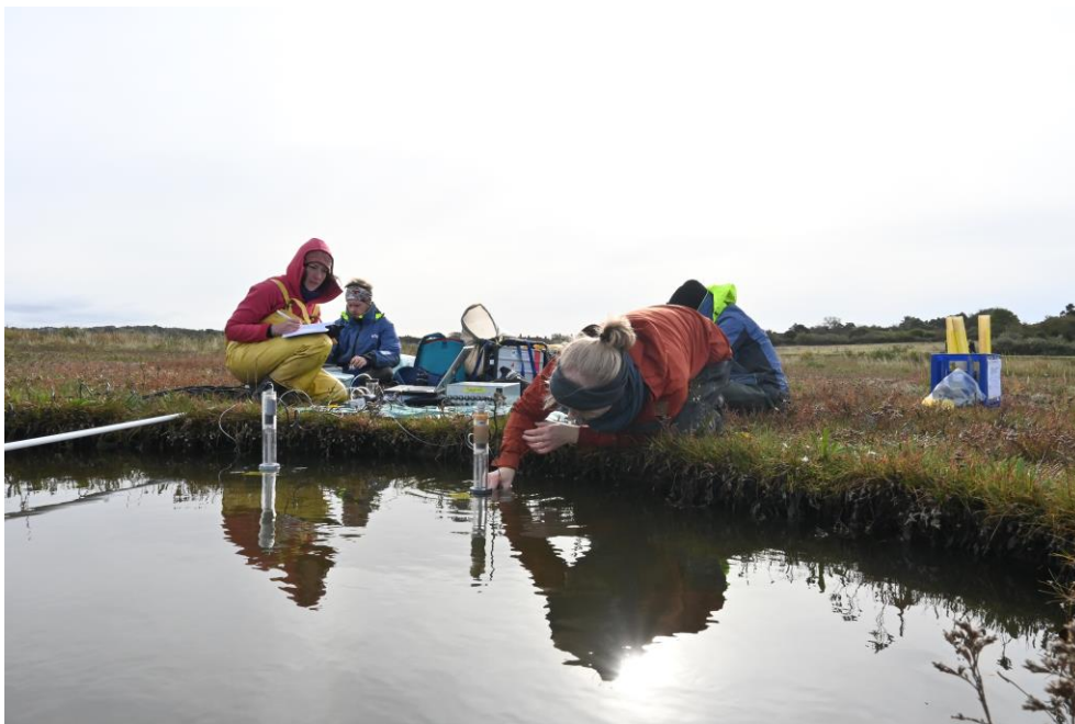
Figure 2 Installation of incubation chambers for measuring sediment-water fluxes of dissolved compounds.
