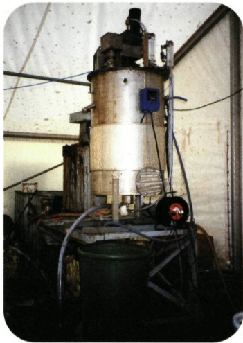
Fig. MIT 2: In this Biometal sludge reactor (BMSR) special bacteria are mixed with soil contaminated with heavy metals. The metals are linked to the biomass, which is removed from the process water after settling of the soil.
