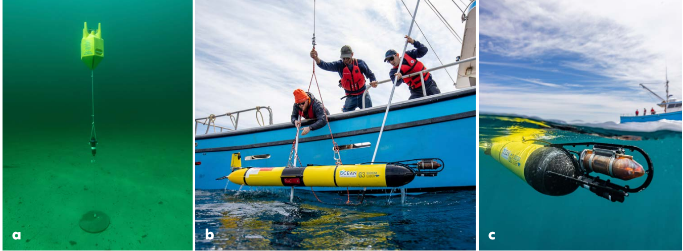
FIGURE 3. (a) Deployed acoustic receiver mooring (with sacrificial disc anchor, acoustic release, and yellow flotation collar housing the acoustic receiver) before deployment. (b) Recovery of a Slocum electric glider fitted at the bow with a Digital Acoustic Monitoring (DMON) external hydrophone to record whale calls. (c) Close up of DMON. Photo credits: Nicolas Winkler Photos courtesy of the Ocean Tracking Network
