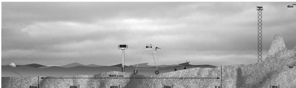
Fig. 11. Schematic layout of a monitoring/measuring programme. From left to right: buoy, frame, pole, WESP, sledge, ARGUS tower, dune. In deep water, wave boundary conditions are measured by a buoy, while in shallow water, waves and water levels are measured from a pole. WESP and ARGUS monitor depths and heights. An instrumented sledge and a frame perform experimental process measurements.
