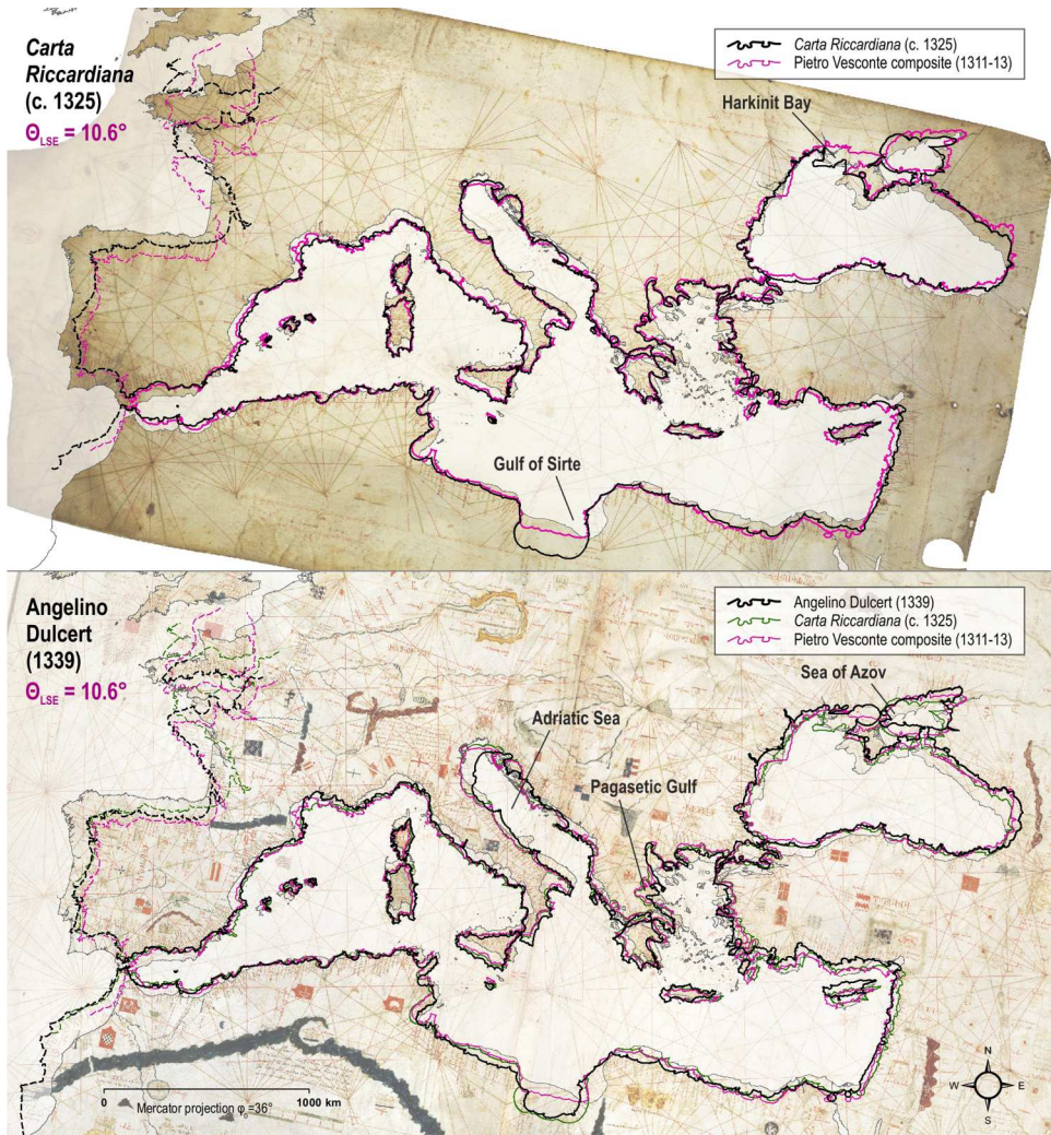
Figure 2. The overlay of the Carta Riccardiana (c. 1325) and its vectorized coastline (the upper part) and the overlay of Angelino Dulcert's 1339 chart and its vectorized coastline (the lower part) with the vectorized coastlines of some of the earlier-made portolan charts. Chart sources: Biblioteca Riccardiana , Ricc. 3827.; Bibliothèque nationale de France , GE B-696 (RES). Basemap shapefile source: mariner-egions.org (Claus et al., 2017).
