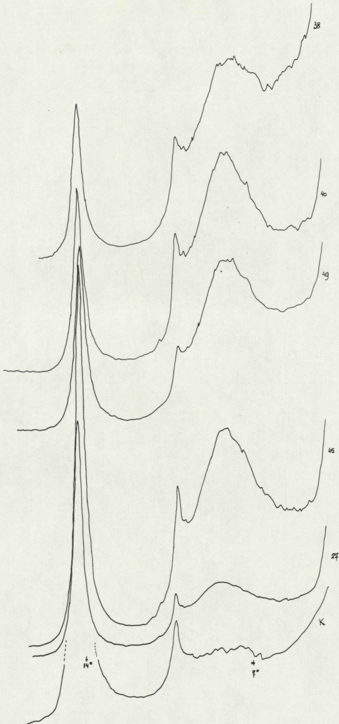
Fig. 4. X-ray diffraction patterns of oriented samples at lower pressure (ca 5 mm Hg).
