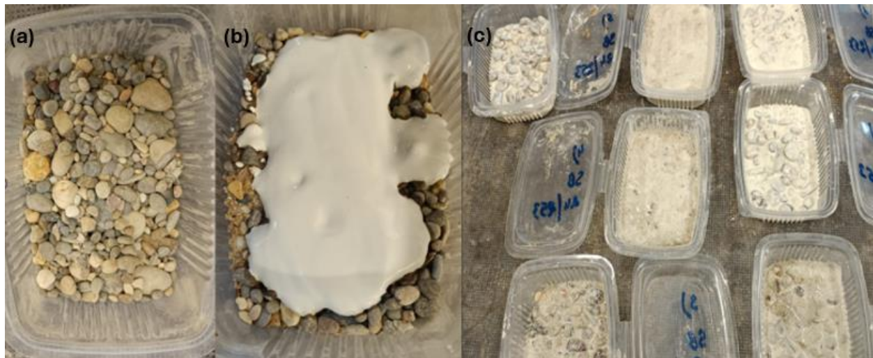
Figure 3 Steps to prepare samples for surface texture influence: (a) Prepare concrete samples with varying aggregate sizes. (b) Pouring the binder mixture over the aggregates. (c) Compaction of the samples using vibration.
