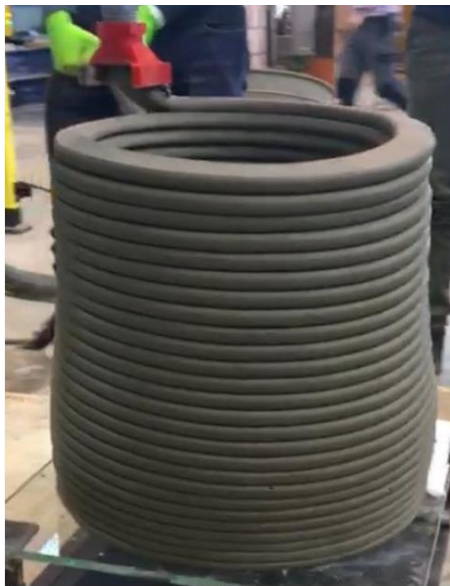
Figure 5: An example of 3D printing of an outer shell [10]
